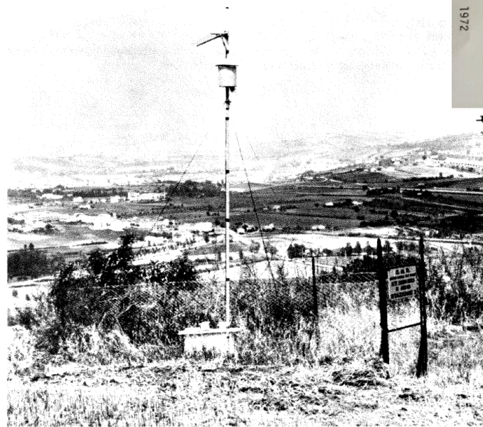
Fig. 4 - The lodging of a seismic outstation.
